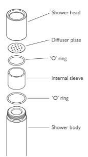
The diffuser plate should never require removal, but should the holes in the diffuser plate become blocked please see below:
