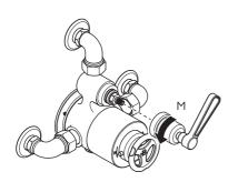
I Remove the lever assembly (M) by fully unscrewing in a counter clockwise direction. We recommend wearing a rubber glove such as those used for washing up to improve grip.
