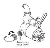
3 Unscrew the elbow assemblies from the sides of the thermostatic valve body.
