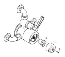
2 Remove the override (C) and temperature stop (D) by unscrewing and removing screw (E). Fitting handwheel (A) and set screw (B) will aid with removal of override (C).
