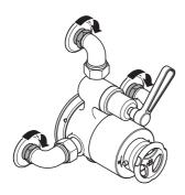
2 Support the thermostatic valve. Unscrew the three collar nuts in a counter clockwise direction. This will release the thermostatic valve from the mounting surface.
