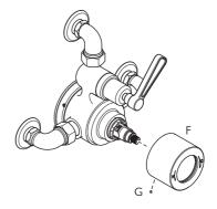
3 To remove the thermostatic cartridge cover (F) unscrew the set screw (G) using a 1.5mm hexagonal key and pull the thermostatic cartridge cover away from the valve body.
