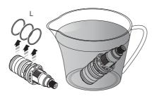
5 Check the 'O' rings (L) for damage (ie. cuts or tears). Remove the 'O' rings before soaking the cartridge in descaling fluid. Soak the cartridge according to the instructions on the descaling fluid packaging. Rinse under cold water before fitting (refer to the 'installing the thermostatic cartridge' section to install).
