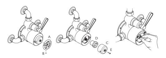
Remove the thermostatic control handwheel (A) by unscrewing set screw (B) using a 2mm hexagonal key.
