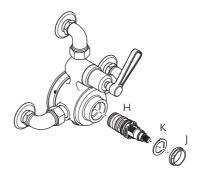
4 To remove the thermostatic cartridge (H), unscrew and remove locking nut (J). Remove anti-rotation washer (K) and pull out cartridge. To help with cartridge removal, it is recommended you fit override (C) with screw (E) to make pulling the cartridge out easier.
