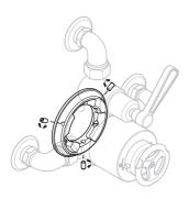
I Isolate the hot and cold water supplies before the shower valve. Unscrew the three set screws from the valve backplate.
