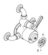
I Isolate the hot and cold water supplies before the shower valve. Remove the thermostatic control handwheel (A) by unscrewing set screw (B) using a 2mm hexagonal key.
