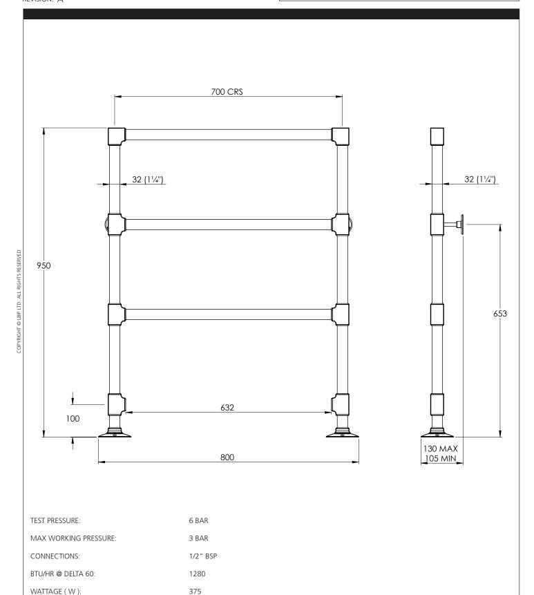
THIS LEFROY BROOKS RAIL IS SUITABLE FOR BOTH OPEN AND CLOSED CIRCUITS
