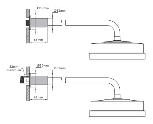
5 The shower arm connector can be adjusted within the wall opening as shown above.
