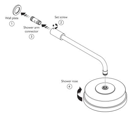
To aid installation and prevent damage, the shower rose and arm can be disassembled as below.
