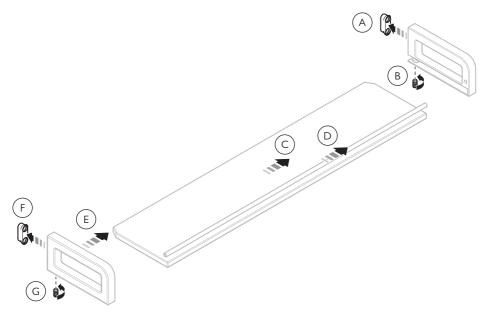
Shown with right hand bracket secured in place first
