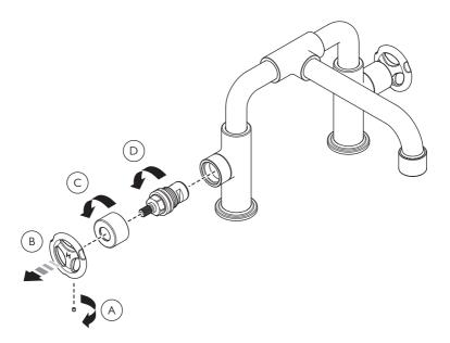
Before continuing please ensure that the water supplies have been isolated and drained where necessary.
