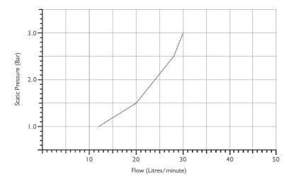
Note: Balanced pressures shown are applied directly to the hot and cold inlets; flow rates indicated are free flowing and may vary subject to restrictions created by installation, pipework, layout or application.
