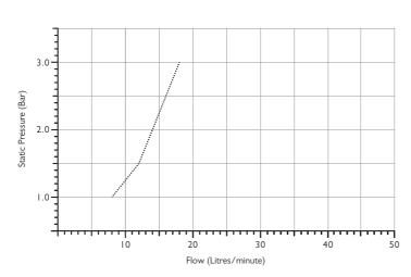
Note: Balanced pressures shown are applied directly to the hot and cold inlets; flow rates indicated are free flowing and may vary subject to restrictions created by installation, pipework, layout or application.
