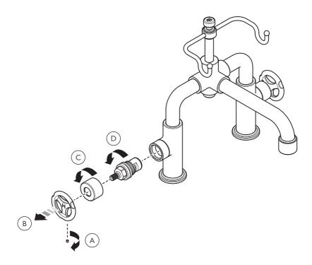
Before continuing please ensure that the water supplies have been isolated and drained where necessary.
