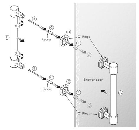
Note: Before fitting the handles ensure that rubber 'O' rings are fitted to the components in contact with the shower door. These are factory fitted, though may have worked loose during transit. Fitting the handle without 'O' rings in place may damage the shower door.
