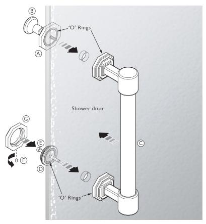
Note: Before fitting the handle ensure that rubber 'O' rings are fitted to the components in contact with the shower door. These are factory fitted, though may have worked loose during transit. Fitting the handle without 'O' rings in place may damage the shower door.
