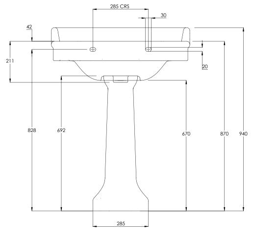
ALL SHOWN DIMENSIONS ARE IN MILLIMETERS AND ARE SUBJECT TO STANDARD CERAMIC TOLERANCES.
