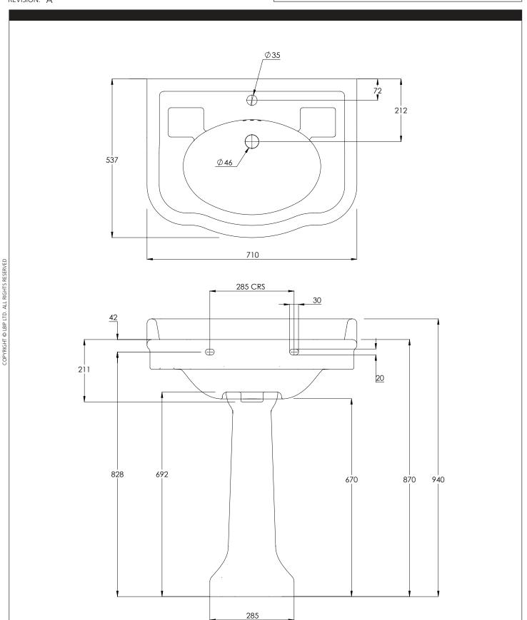
ALL SHOWN DIMENSIONS ARE IN MILLIMETERS AND ARE SUBJECT TO STANDARD CERAMIC TOLERANCES.
