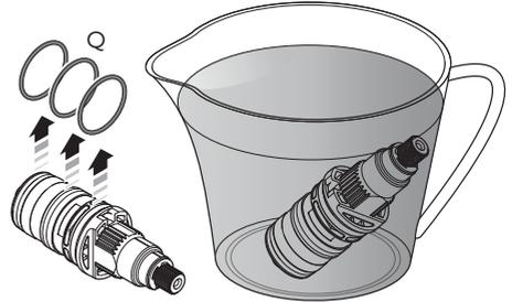
8 Check the 'O' rings (Q) for damage (ie. cuts or tears). A set of three replacement 'O' rings are available (PTS027). Remove the 'O' rings before soaking the cartridge in descaling fluid. Soak the cartridge according to the instructions on the descaling fluid packaging. Rinse under cold water before fitting (refer to the 'installing the thermostatic cartridge' section to install).
