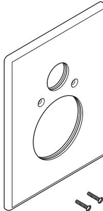
PTC036 – Facing plate including gasket, screws and 'O' rings (GD & BL models only)
