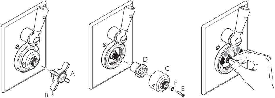
Remove the thermostatic control cross handle (A) by unscrewing set screw (B) using a 1.5mm hexagonal key.
