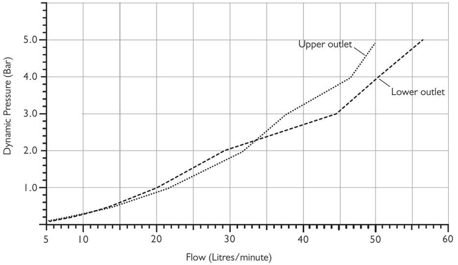
Note: Balanced pressures shown are applied directly to the hot and cold inlets; flow rates indicated are free flowing and may vary subject to restrictions created by installation, pipework, layout or application. The outlet temperature during testing was 38°C.
