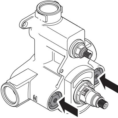
6 Isolate the hot and cold water supplies as follows: The non-return valve covers have a screw in the centre. Use a screwdriver to turn the screws in a clockwise direction until they reach their stop. Do not over tighten the screws as this may damage the non-return valves.
