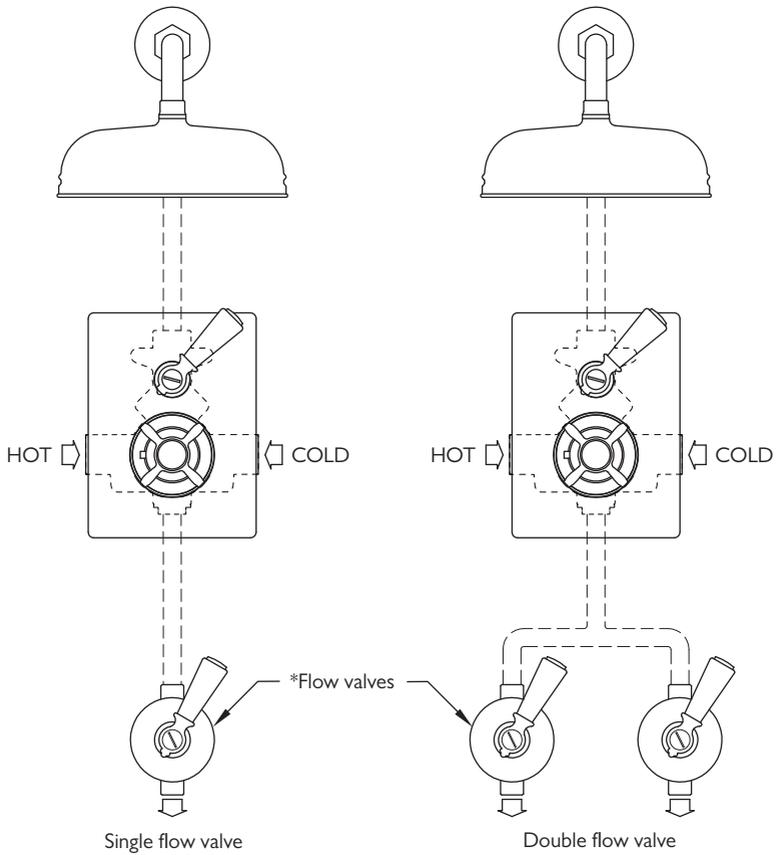
For adding a hand shower, body jets or bath filler, remove the  $\frac{3}{4}$ " BSP plug from the bottom of the valve body and connect suitable flow valve(s).
