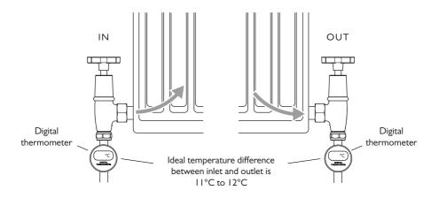
Note: On/off & lockshield valves can be fitted either side of the radiator
