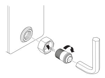
Apply suitable sealant or tape to the threads of the adapter.
