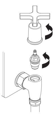
To replace or clean the cartridge within the radiator valve unscrew the cross handle/handwheel assembly. Wearing a rubber glove such as those used for washing up will improve grip. The cartridge can be unscrewed and removed using a 17mm spanner or socket. When finished, always check for leaks.
